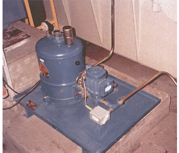
The Portland Rotating Oven is driven by FLS Gear equipped with a CJC™ Filter for retaining particle, oxidation and water from the gear oil.
