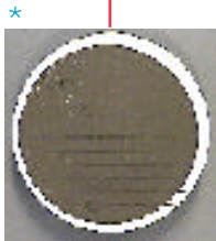
Oil sample analysis taken from a sump with normal on-line filtering.
