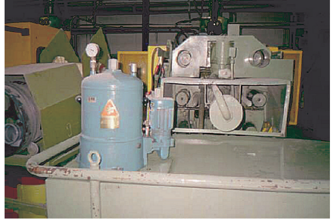
At Wavin Metalplast in Buk, Poland all STORK plastic injection moulding machines are equipped with CJC™ Fine Filters.
