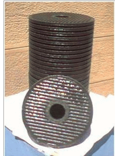
Filter element type B 27/54 after 1.212 hours of continuous operation in Symons no. 3 at Compania Minera Disputada
